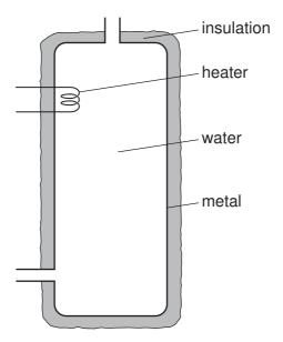
Water at the bottom of the tank stays cold for some time.
